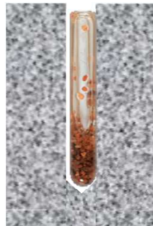
Insert Spin In Capsule with air bubble nearest to surface of concrete
